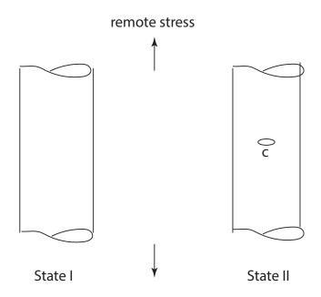
$$\Delta G = G_{II} - G_I = +2\gamma_F \pi \left(\frac{c}{2}\right)^2 - \frac{4}{3}\pi \left(\frac{c}{2}\right)^3 * \frac{\sigma^2}{2E}$$
