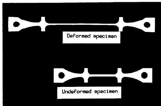
Fig. 1. Superplastically elongated specimen of Y-TZP at 1450°C.
