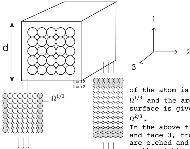
(Figure 1) Now we consider the etching of atoms from faces 2 and 3, and depositing those atoms on face 1, as shown below.
