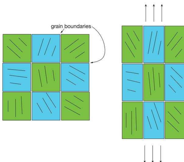
(Figure 4) The figure on the left shows the deformation of a polycrystal. Each crystal deforms in the manner discussed in the previous section, but in a way that is compatible with other crystals surrounding it.
