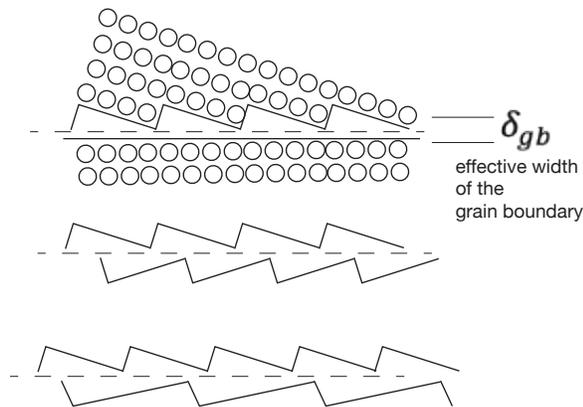
(Figure 6) Notes: (i) Any misorientation between the crystals will necessarily give rise to ledges as the boundary. (ii) The ledges may be further apart or closer in as contrasted in the bottom two drawings. (iii) In the top picture one crystal is shown to be flat. However, a change in the plane of the boundary can introduce ledges in the bottom crystal.
