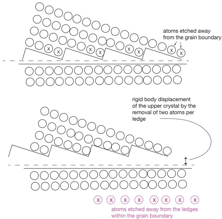
**Figure 7:** Etching of atoms out of the boundary at ledge sites. As a result the two crystal move closer together as rigid bodies.
