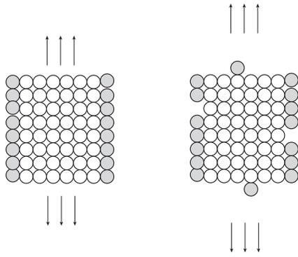
(Figure 3) In this instance we move two atoms (total) from the transverse faces to the face to which we have applied a tensile stress. The tensile strain will now be given by Eq. (1) but weighted by a factor that is equal to two atoms divided by the total number of atoms moved in Figure 2. This weighting factor is equal to
