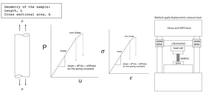
If the cross sectional area is doubled then the load required to achieve the same displacement will double..
