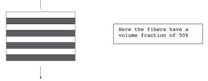
Now the total strain is the sum of the strain in the matrix and the strain in the fibers. Recalling the following relationship between strain, stress, and the E, the Young's Modulus,
