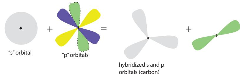
The sp<sub>2</sub> hybridization leads to the planar structure with three fold symmetry. The carbon-carbon bond length in diamond is 154 pm but it is 142 pm in graphite.. can you give an argument for this behavior.
