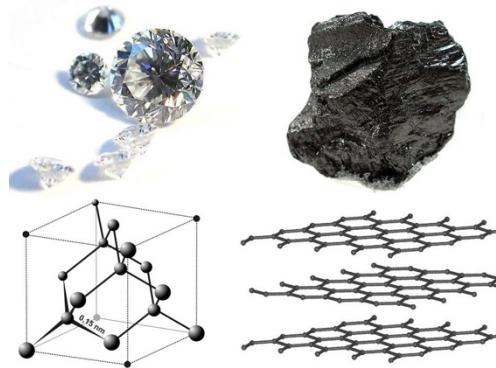
The above is called sp<sub>3</sub> hybridization. Indeed this is the structure of diamond - it has tetragonal symmetry.
