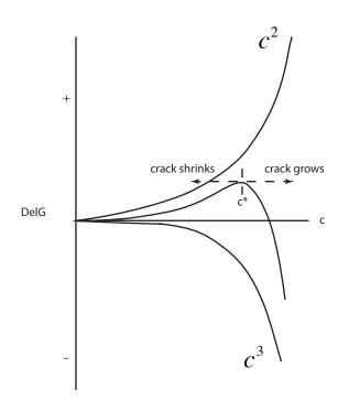
Therefore, the critical condition for fracture is obtained by differentiating Eq. (2.1) and equating it to zero. Which will give the following result:
